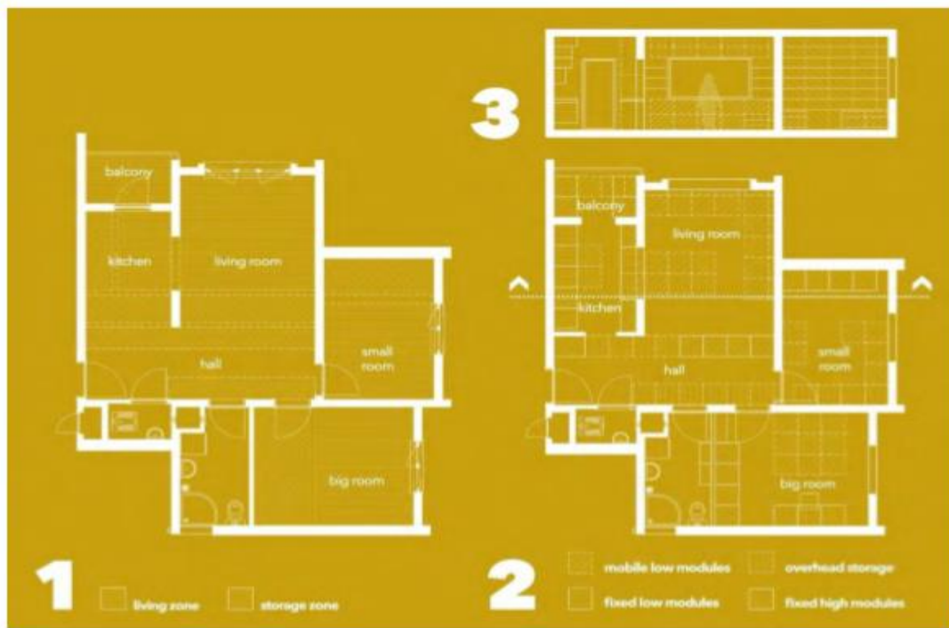
Figure 2. The modular layout showing mobile and fixed module zones and decisions about
