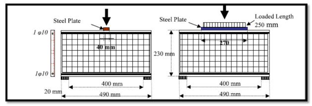
specimens are identified using two abbreviated terms: the first term represents the wire mesh reinforcement type D for Diamond (i.e., expanded), S for Square, C for Chicken (i.e., hexagonal), and R for reference beam (i.e., plain mortar); and the second term represents the mesh opening size (L for large and S for small).
