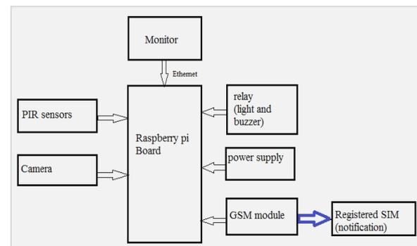
**Fig. (1) : Block Diagram of ATS-IOT**
